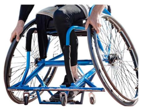
Knee hyperflexion position: This position occurs when the knee angle exceeds 90°, with the feet moving backward. It is made possible by adjusting the sitting angle, as mentioned in the previous items. This position increases turning speed but can cause high muscle tension, affect sitting stability, and influence trunk movements.
